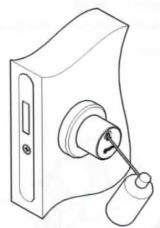
After 10 000 usages, clean contact rolls lightly with lint-free cotton pad. Spray small amount of high quality lock oil i.e. CRC lock oil (with PTFE) onto contact rolls.
